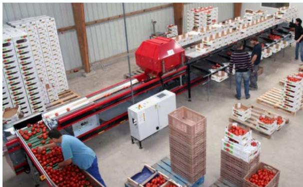
A unique feature of the Pentacup is the patented 5-sided cup. These cups hold products precisely in place, ensuring an accurate weight measurement. Therefore, the Pentacup can sort products with a diameter between 40 and 110 mm (such as tomatoes, kiwis, stone fruit, citrus and apples) with a speed up to 15 cups per second. The lane is equipped with loadcells ensuring accuracy for weight with a maximum std. dev. in weight of 1 %.
