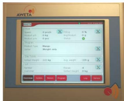
The machine and its operation has been designed to enable easy usage. By using a touchscreen cockpit, the operator has easy access to every program. The user interface enables the operator to walk through the system step by step. Every step eliminates several options, preventing the user to make mistakes, yet guiding him to the necessary decisions.
